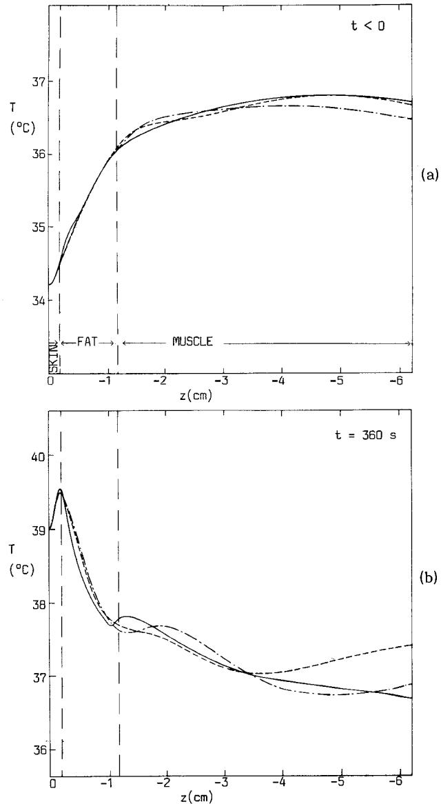
Fig. 1 Retrieval of temperature profiles in a skin-fat-muscle structure irradiated by an electromagnetic wave. The five diagrams from a) to e) refer to the times shown on the respective figures. The curves refer to the profile to be retrieved (continuous line), to the retrieval by using six equally spaced frequencies in the range 1.5-6.5 GHz (dashed line), and to the retrieval by using four frequencies (dotted line) in the same range.
